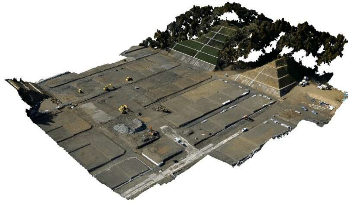
Figure B.1 3D point cloud data created from aerial images (Source: https://www.ad-hzm.co.jp/solution/construction_dx/detail_03/ )
