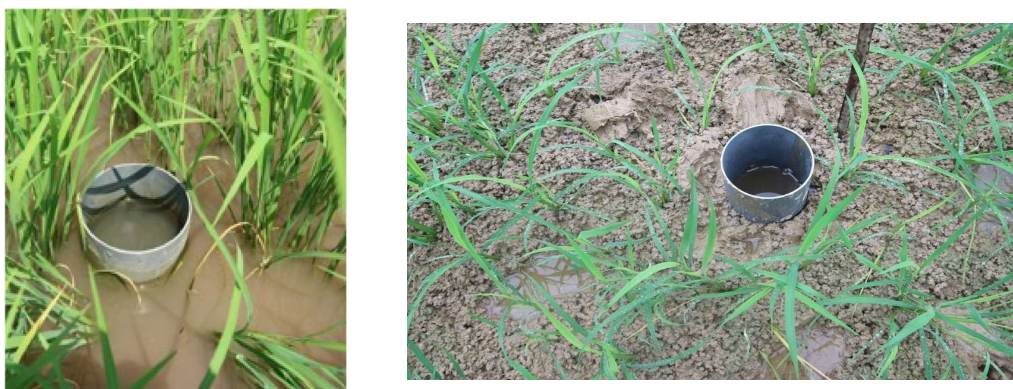
Photo F.1 Simple water depth measurement using PVC pipe
