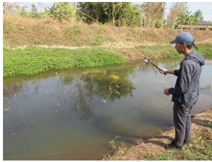
Photo 5.1 Measuring water depth using a fishing line (Left: Thailand, Right: Vietnam)
