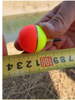
Photo 5.1 Measuring water depth using a fishing line (Left: Thailand, Right: Vietnam)
