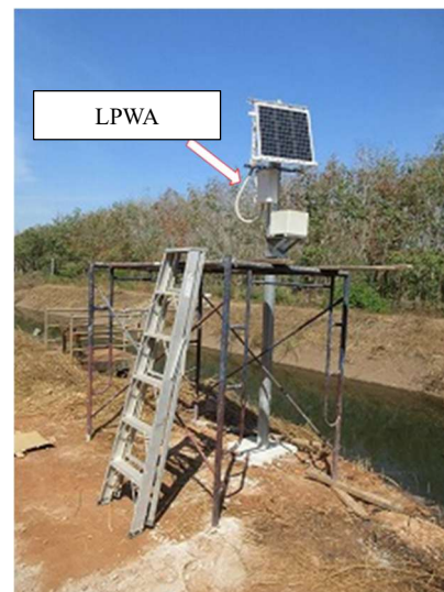
Figure 2.7 Communication control devices. Left: PLC and IoT router (NIRE. 2019), right: LPWA communication device.
