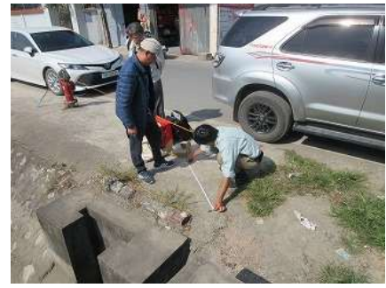
Photo 5.1 Measuring water depth using a fishing line (Left: Thailand, Right: Vietnam)
